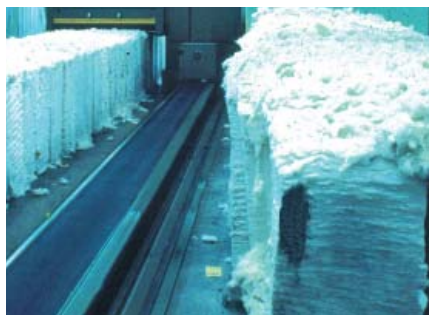
Prevent grease stains from contaminating bales at the gin and during handling as seen on this bale in the opening room of a mill.
